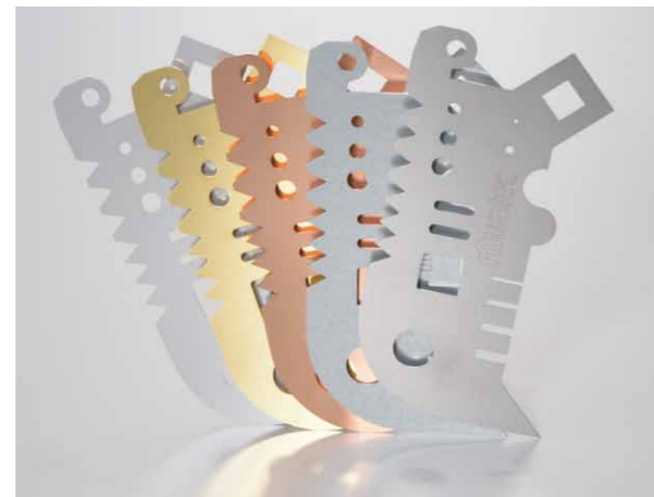
A fiber laser has a wavelength 1/10th that of a CO 2 laser, resulting in a higher laser light absorption rate on metal surfaces.
